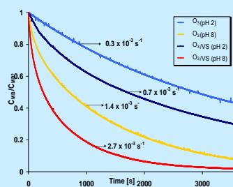
Heterogeneous ozonation, using volcanic sand, enhanced MB removal for each pH level studied. The increased fraction of removed MB could be related to the enhancement of radicals coming from ozone interaction with volcanic sand.
